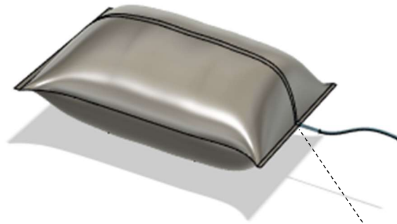
Insert tubing end from air exhaust fitting for airflow measurement
