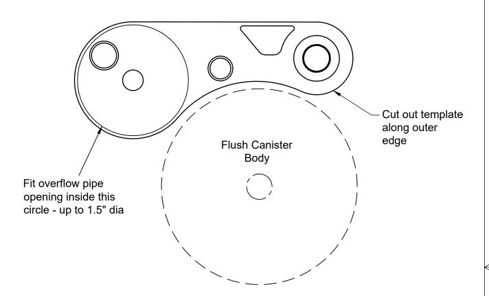
The dual flush style air intake shroud accepts overflow pipe openings up to 1.5" in diameter.
